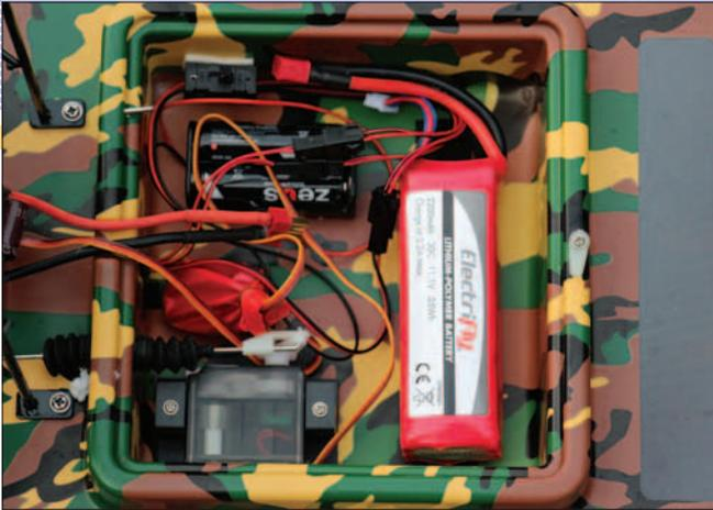
The equipment compartment is quite roomy containing the receiver, steering servo, LED battery and the run pack. (I should mention that the boat is shrouded with this power combination).
