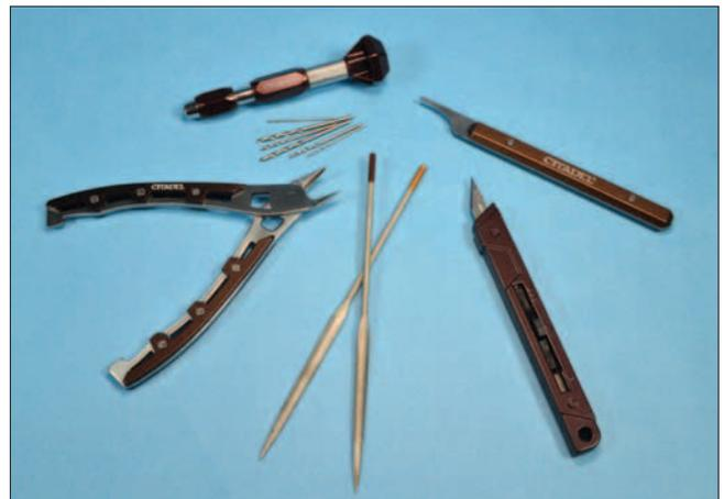
*In addition to model kits for wargaming, Games Workshop offers a complete line of tools to help with the building process. The Citadel Drill has a fine point to enable the modeler to get into tight areas for smoothing parts for assembly.*
