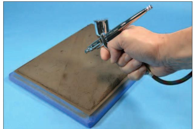
*The Neo TRN1 is a pistol grip, gravity-fed airbrush that can use low pressure to control overspray.* top mounted trigger downward then pulling back for paint spray, the TRN1 incorporates a pistol grip trigger that is pulled back for air pressure then pulled farther for paint release.
