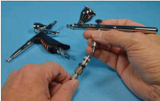
*The Quick Disconnect Set allows airbrushes to be changed without having to turn off the compressor.* Still, I gazed at all the airbrush ads in that magazine, and hoped that one day, I could actually own one of the magical instruments.
