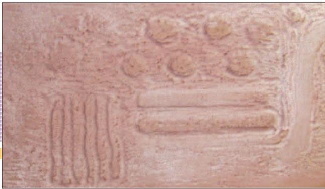
*Pink foam insulation is first cut to size, then various grades of sandpaper are used to give the base some texture.*
