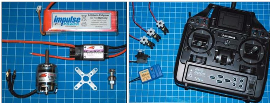
HM's review FW-190 got the full treatment — Impulse 3S 2500mAh LiPo battery, Ultrafly F/18/10 brushless outrunner motor and Apollo Brushless Speed Controller. New 2.4GHz Airtronics RDS8000 RC system was chosen, with three Airtronics 9409IZ Super Micro servos.
