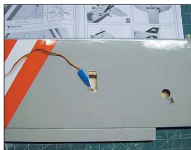
*Self-aligning horizontal stabilizer and vertical fins are installed with 6-minute epoxy. Snaking the leads for the aileron servos is effortless thanks to two lengths of string that come factory installed in the F-14 TAMEcat's one-piece wing. Servo bays are factory cut.*
