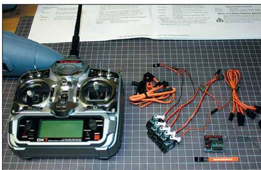
*Recommended RC system is Spektrum 2.4GHz with three to six E-flite S75 servos, assorted extensions and Y's.*
