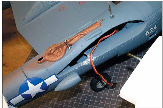
*Each wing panel mates to a fuselage boom and secures with two plated Phillips-head screws.*
