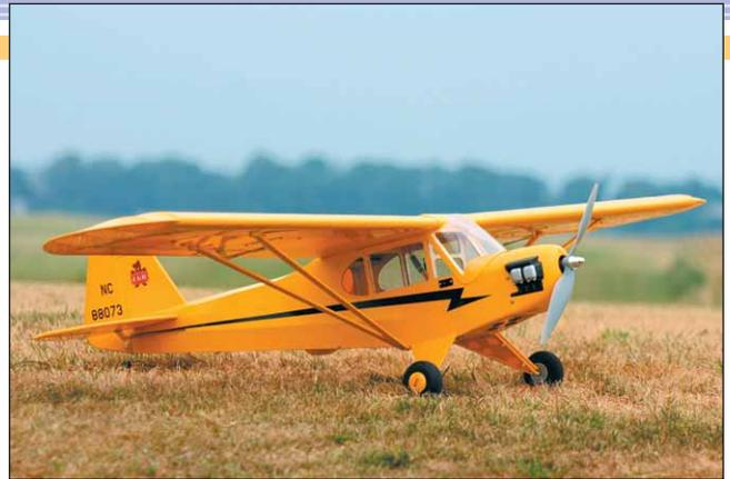
*Conventional landing gear and steerable tailwheel come with the kit. Ground handling is excellent, even on grass runways.*
