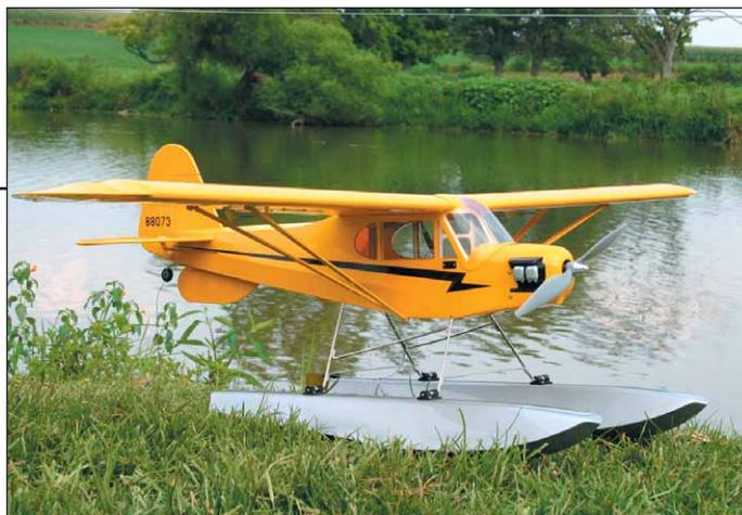
Assembly goes quickly, although the conventional landing gear steps were held off until the model could be flown on floats. For this, E-flight offers a complete 25-Size Float Set. The molded fiberglass floats come factory assembled and painted in silver, making them look a lot like the popular full-scale Edo floats. Mounting equipment, water rudder and connecting linkage are all provided in the float kit, which is recommended for the new Ultra Stick 25 as well as the J-3 Cub 25 ARF.
