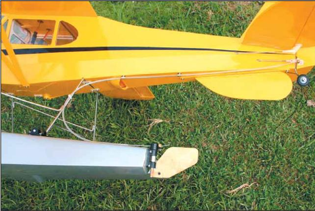
*Water rudder and dorsal are mechanically linked to rudder horn. Entire float assembly can be removed in a few minutes.*
