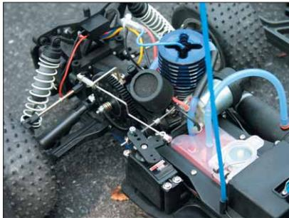
*Traxxas' Pro .15 engine and tuned pipe make more than adequate power for the 2WD Nitro Sport. EZ starting is quick and pretty much effortless.*
