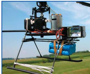
*E-flite's Blade CP electric helicopter is 100 percent factory assembled and tested. Just charge the Ni-MH motor pack and fly. The model's factory-installed six-channel RC system has a built-in gyro and electronic speed control, and the transmitter features idle up and CCPM mixing. The 9.6-V 650mAh Ni-MH pack is included.*
