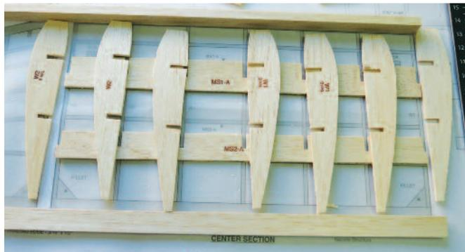
*Starting with the wing's center section, all of the pieces were separated from the carrier sheets and were dry-fitted in place before any glue was used. This makes any minor trimming much easier to do than if there are blobs of wet cement all over the parts being installed.*
