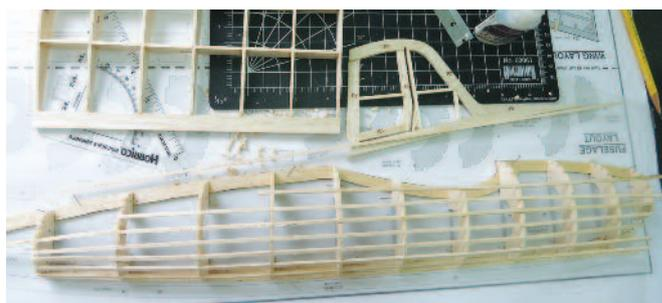
*At this stage the stringers have only been dry-fitted, as for a straight build they must be installed in opposing pairs to prevent warpage, but it's still pretty easy to see how the stringers begin to give the fuselage shape and dimension.*
