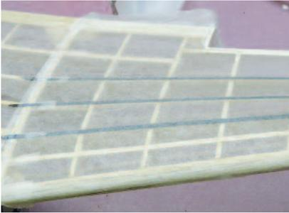
The DC-3 is engineered primarily as a display model, so to convert it to a flying model requires a bit of strengthening. To do this without adding much weight, strips of carbon fiber were adhered in place.
