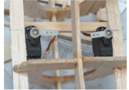
For ease of installation and future maintenance along with helping to achieve balance without the addition of unnecessary weight, the servos were mounted as far forward in the fuselage as practical.
