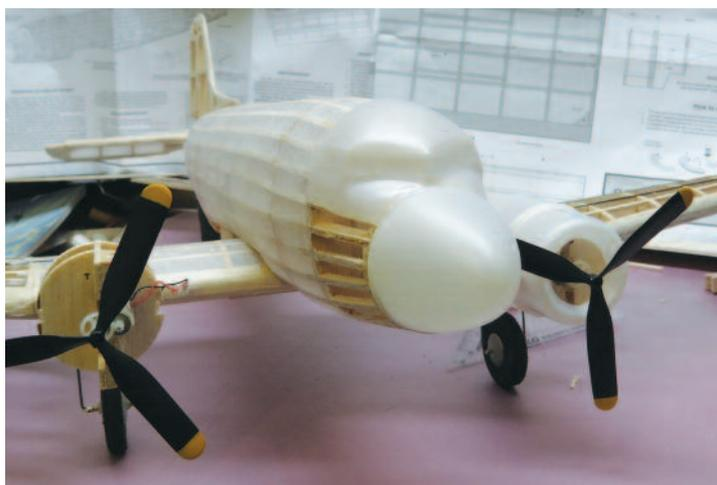
*Due to the numerous compound curves present on the DC-3 it needs to be covered in sections, but the instructions that come with the kit describe the process in detail and will walk the builder through the process.*
