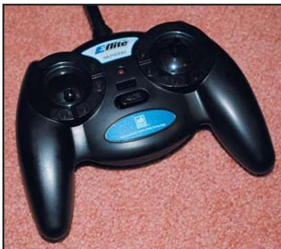
*ance. Double-pushbutton, electronic trims are present on all four channels. The transmitter requires only four AA alkaline cells, and they are included.*
