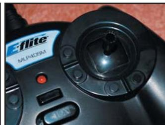
*E-flite Blade mCX transmitter uses Spektrum DSM 2.4GHz technology for interference-free, crystal-free and worry-free guidance.*
