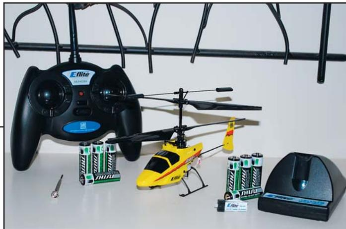
The Blade mCX — with the “m” for micro — is a reduced-size version of the enormously successful Blade CX coaxial, contra-rotating, twin-rotor trainer. The rotor span is just 7.5 inches, and the entire model, battery installed and ready to fly, weighs only one ounce. It’s a truly amazing design and production accomplishment.
