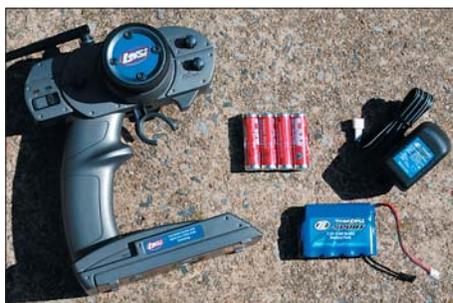
Losi 2.4GHz pistol-grip transmitter and alkaline batteries are included in the set, as are the onboard motor battery and AC charger. Note heavy-duty steering servo.
