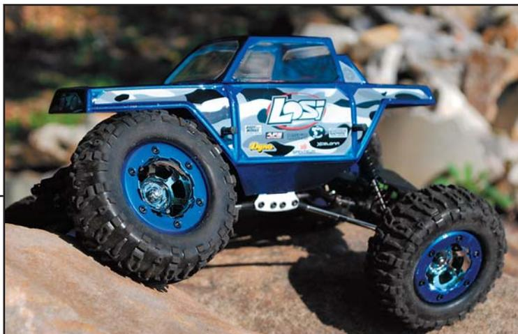
The twin vertical-plate chassis design is ideal for rock crawling, yielding tons of clearance and maximum suspension travel. The suspension is a multi-link design, with metal lower links and plastic upper "Y" links for maximum travels and good ground clearance. It also has extra-long-travel, oil-filled shocks to maximize suspension movement and get the axles over surprisingly large obstacles with no problem.
