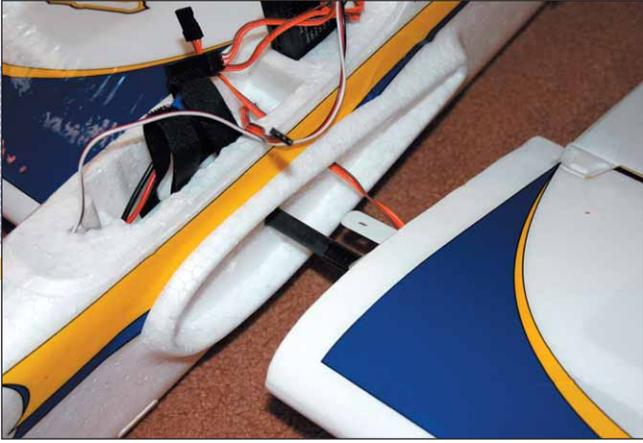
*Wing panels plug in over carbon joiners for strength, easy transportability, and rapid field assembly and breakdown.*
