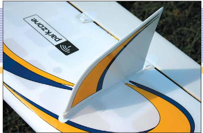
*Press-in upper and lower side force generators can be installed or removed in seconds. Secure to the mounts with clear tape. RC works flawlessly, and pilots can shuttle between high and low rates with a flip of a transmitter switch.*
