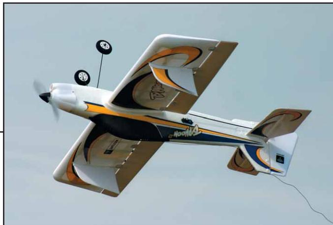
maneuvers, and their deflection is more than adequate. The surfaces are hinged with a unique pin & snap-clip system that actually works very well.
