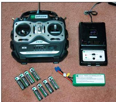
2 3D comes with an installed electric power system, a LiPo pack and charger, transmitter batteries and a complete, factory-installed ZX10 FM radio system.
