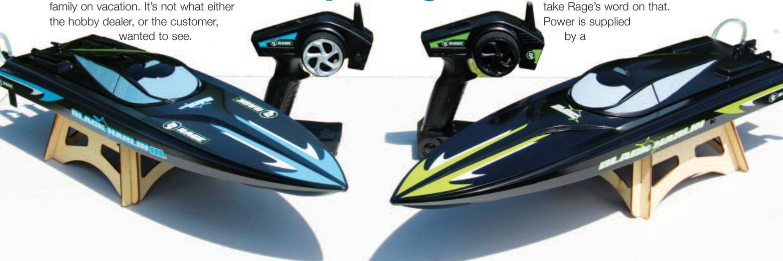
7.4V 1500mAh Lithium-Ion battery and the package includes a USB style charger for the battery pack. Also included with the boat is an extra propeller, a length of hook-and-loop material for securing extra battery packs a hex wrench for servicing the prop shaft and a really handy wood display/service stand. The transmitter is a full-size wheel type and has all the necessary forward and reverse switches along with trim centering. Considering the price point, this is a nice package.
