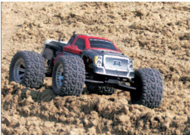
The suspension is able to articulate and keep the tires in contact with the surface in the roughest of conditions.
