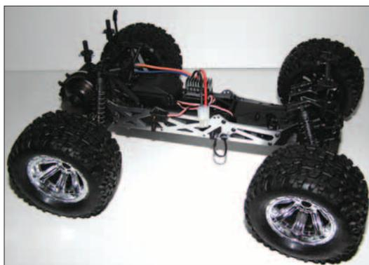
Left: All of the components are attached to the TVP (Twin Vertical Plate) chassis which is formed from 2mm thick stamped aluminum. Right: The ATX300 transmitter is brightly colored and features a steering wheel that can be adjusted in six positions for either right or left handed users.
