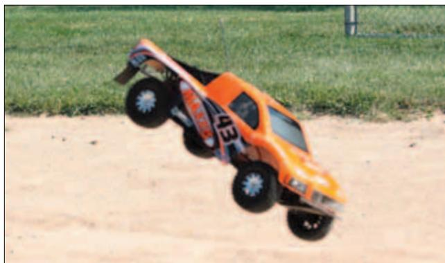
*The Blitz is capable of jumping over any number of obstacles and landing without damage. The nose down attitude shown here was adjusted by moving the battery from the front to the rear of the battery tray. This made landings after the jump more horizontal.*
