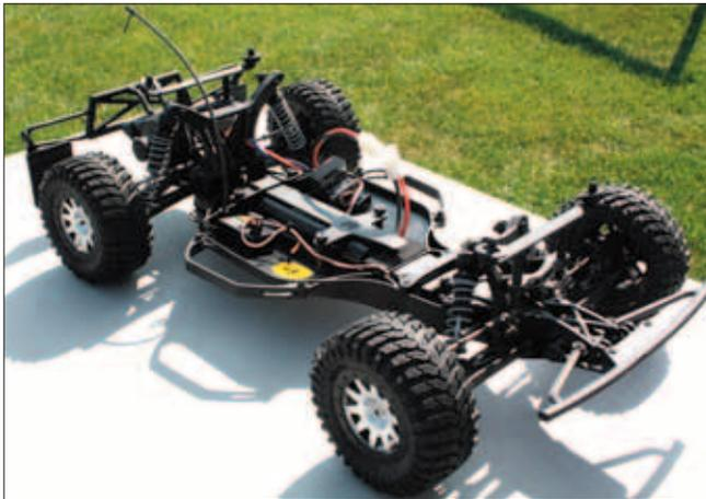
*The Blitz chassis is a molded composite design with plenty of extra webbing used in high stress areas for strength and resistance to flexing.*
