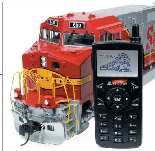
The transmitter stands proudly beside Aristo-Craft's Dash Nine with a receiver installed. Transmitter and receiver work together to move this fifteen pound beast around the layout with easy chair reliability.
