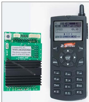
The receiver image on the left has been magnified to give you a better view of it. The transmitter shows the operating screen, with "C-44" being the locomotive and "600" being its cab number. This is Single Unit Cab-0, the speed is "0" and the direction is forward.
