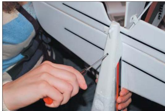
*Plastic studs under the fin pass through the stabilizer and fuselage. Two Phillips-head screws secure the entire tail section.*
