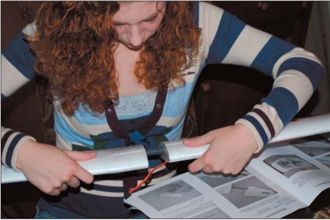
*Devin Troy slides the wing panels together over the carbon joiner. Two ABS covers secure the panels.*
