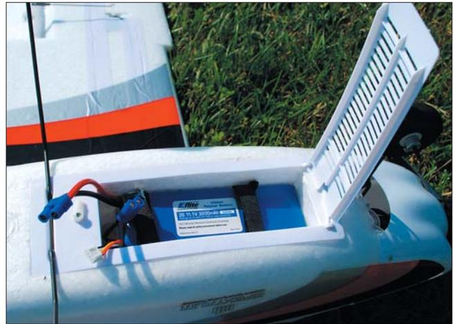
*Battery access is through a sturdy door beneath the fuselage. Two hook & loop band hold LiPo securely.*
