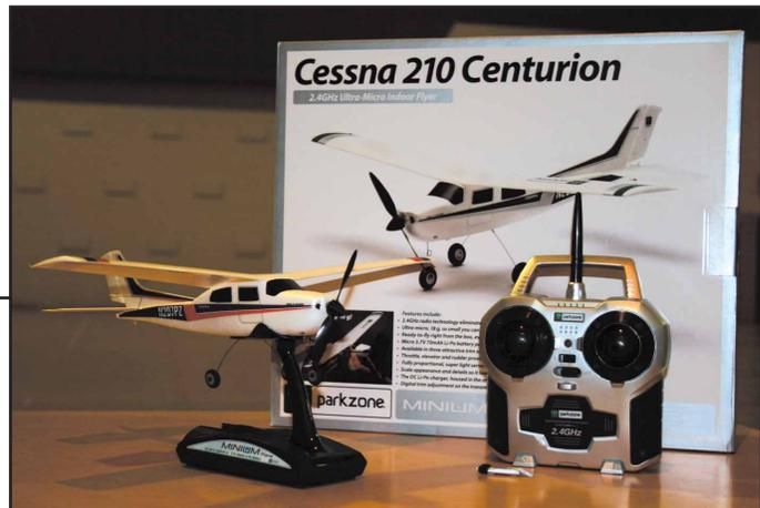
percent ready to go, so setup takes only a few minutes. I inserted four AA batteries in the transmitter, then the other four in the stand-charger, then slipped the tiny LiPo cell into the slot at the front of the charger. The charger's LED glows solid red while the cell charges, then begins to blink as the cell nears capacity. When the charger blinks once every 20 seconds, the cell is ready to go.
