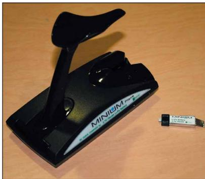
Two AA batteries power the quick charger that's built into the Cessna's display stand. Just insert the 3.7V 70mAh LiPo flight cell and the LED glows solid red. The LED will blink every 20 seconds when the charge is complete.
