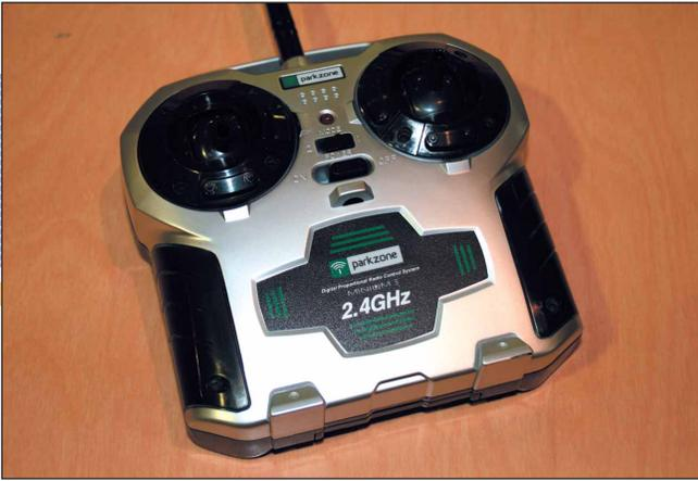
*Three proportional channels handle elevator, rudder and motor speed. 2.4GHz technology assures interference-free flight.*
