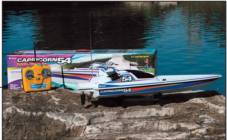
Once at the pond, I prepared the transmitter by screwing in the antenna and inserting the six alkaline cells in the battery tray. Next, I removed the battery access hatch from the deck by removing the two retaining spring clips, then I slid the battery into the mounting slot. Hook & loop is factory applied, and holds the battery in position, but not so firmly that it's hard to remove; the pack actually comes free with very little pressure.
