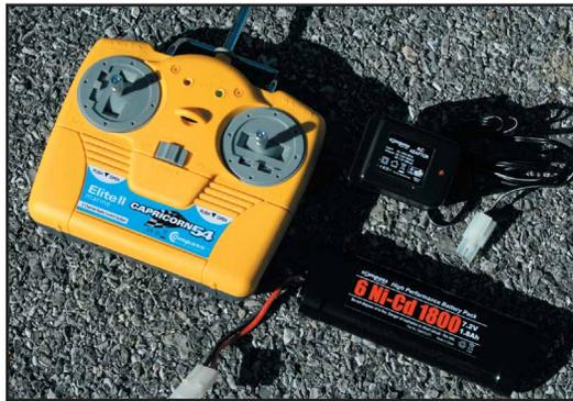
A complete 2-channel RC system comes factory installed. Capricorn 54 also comes with an 1800mAh 7.2-volt NiCD battery and AC charger.
