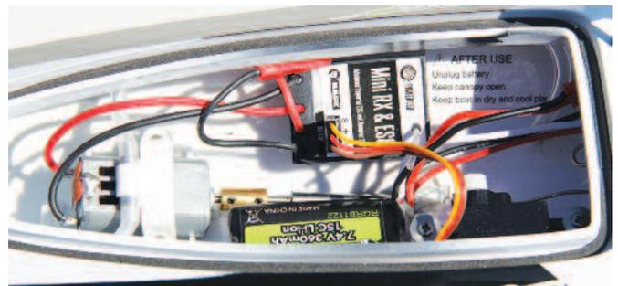
Listed in the manual as waterproof, the electronics are neatly packaged within the hull and protected by a soft, thick gasket that does a good job of keeping water out. The boat also includes the hex wrench needed to loosen the set-screw that holds the prop shaft to the coupling, so maintenance is trouble free as well.
