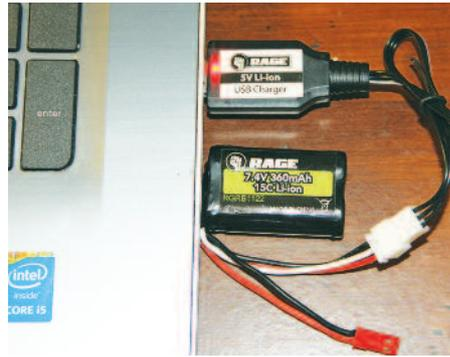
The included 7.4V lithium hull battery offers an acceptable eight minutes of run time and is charged via the now standard USB port.
