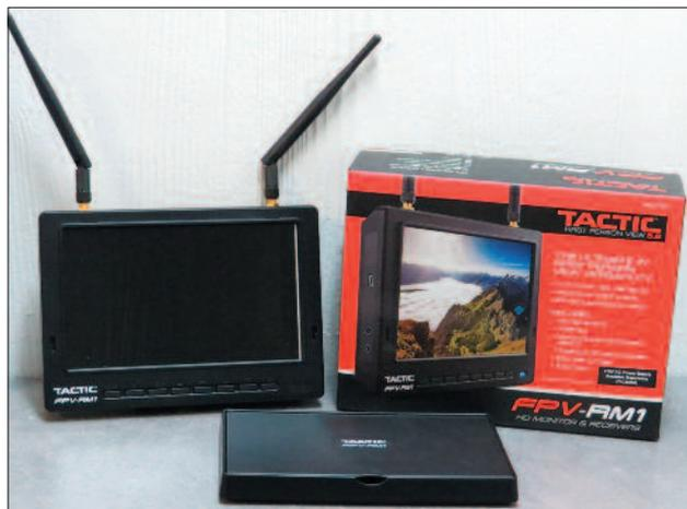
*The seven inch monitor offered by Tactic includes two antennas, sun shade and a built in battery.*
