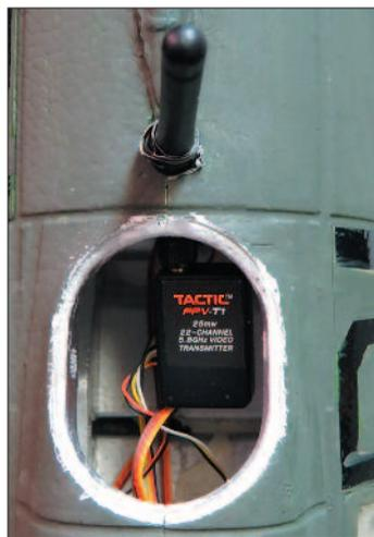
*Mounting the system was easy. The size of the FPV transmitter requires minimum space, and for a unique view, a security camera was mounted in the ball turret.*
