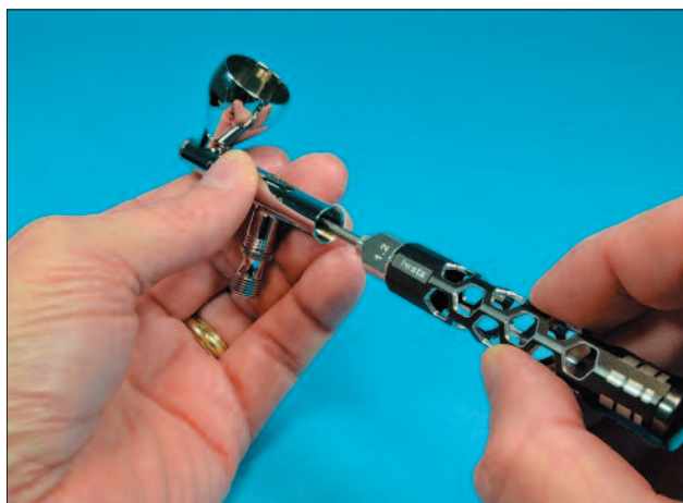
The Needle Packing screwdriver is a highly specialized tool used to replace the packing seal in the airbrush body.
