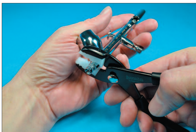
The soft nose pliers can grasp almost any size nozzle cap securely and can safely remove the cap without any damage.
