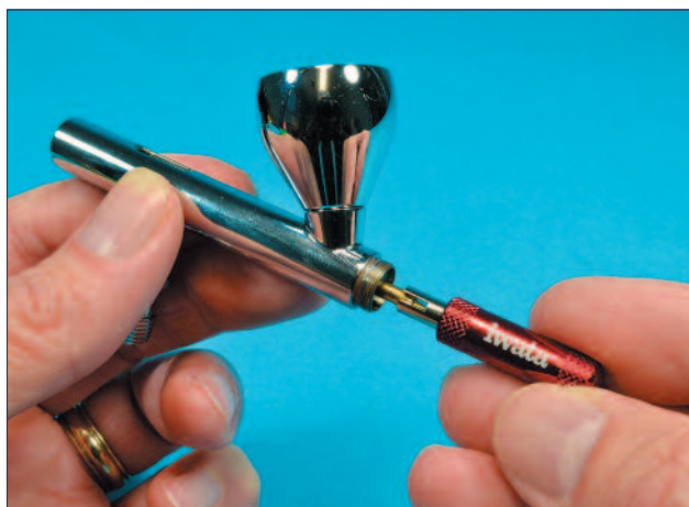
The nozzle wrench allows the tiny paint nozzles to be removed without the risk of stripping the threads.
