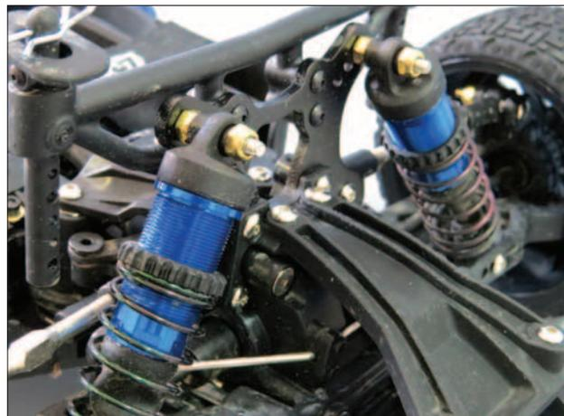
*The vehicle is equipped with adjustable aluminum shocks which keep the tires firmly planted.*
