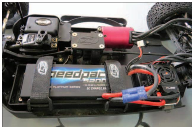
*All of the testing was done using a Dynamite 5200mAh 2S lithium battery pack for juice.*
