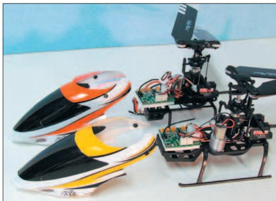
*The canopies of the Heli-Max helicopters are brightly colored to aid in orientation.*
