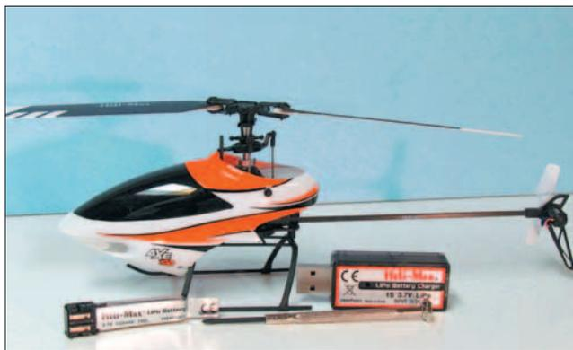
*The 100FP differs completely in design from previously released fixed-pitch helis as it shares the same rotor blades as the collective pitch version.*
