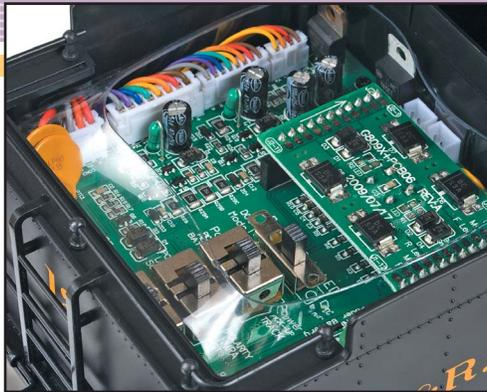
*Pop off the coal load and underneath is this tidy and well-designed power board. The clear plastic shield keeps any condensation that forms inside the coal load from dripping onto the power board.*
