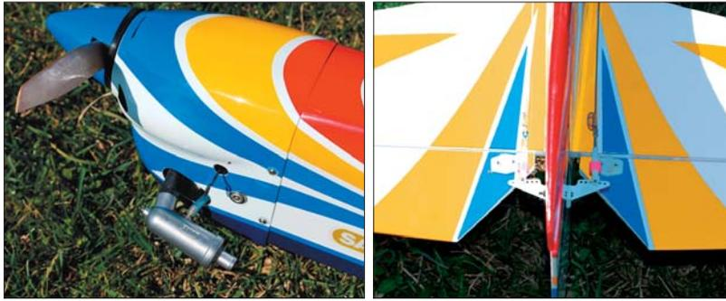
*Perfect cowl cutouts are possible thanks to the clear plastic dummy cowl that comes with the kit. When the clear cowl is right, just trace the openings onto the factory-painted, fiberglass cowl. Complete hardware for the pull-pull rudder is included.*
