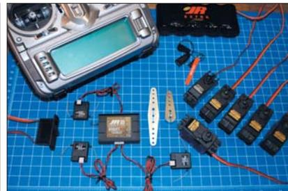
Hobby Merchandiser's review model is equipped with an Evolution 50GX gasoline engine and an Evolution Wraparound Muffler. RC system is a JR 12X with a JR R1221 receiver and three remote receivers, and a 5-cell 3000mAh battery. Servos are four DS8411, a DS8717 for rudder and a DS821 for the throttle.
