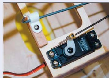
Standard-size, no-frill digital servo is fine on the throttle for intermediate sport pilots. Experts will demand a faster servo for hot 3D response. Plywood servo tray allows mounting on either side of the fuselage.
