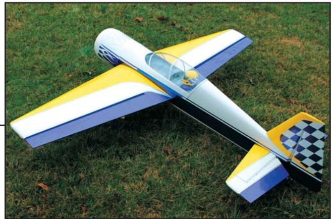
I selected four JR DS8411 servos for the elevators and ailerons, and a DS8717 for the rudder. Since my piloting reflexes are not any faster than a standard digital servo, I felt that the DS821 would be fine for throttle. A JR 5-cell, 3000mAh battery powers the onboard system.
