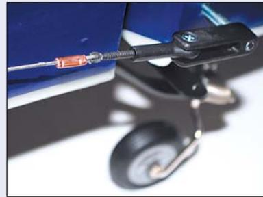
The YAK 54 rudder can be set up for pull-pull control with the servo in the RC bay, or the rudder servo can be mounted at the tail for use with a turnbuckle pushrod like the elevators
