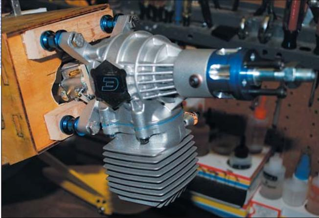
The Evolution 50GX installs easily, although a bit of ingenuity is certainly helpful. Evolution 20mm Spacers position the engine correctly for propeller clearance, and the firewall must be relieved behind the wooden spacers for carburetor clearance.
