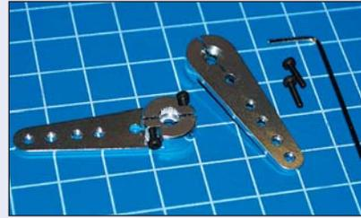
Slop-free linkage is mandatory for a large aerobat like the YAK 54. JR 1-1/2-inch Single Servo Arms (JRPA236) and 3-inch Double Arms (JRPA237)
