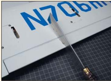
Flaps are separated from the ailerons with a fine-tooth Zona saw. Factory construction allows for separation by cutting through the leading and trailing edges of the ailerons. Side-by-side ribs make the modification neat and easily accomplished. Care must be taken to prevent cutting into the trailing edge of the wing.
