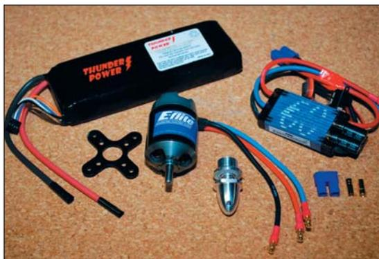
HM's Pawnee uses E-flite's Power 25 Brushless Motor, 60-amp ESC and 11.1-volt 4200mAh LiPo battery.
