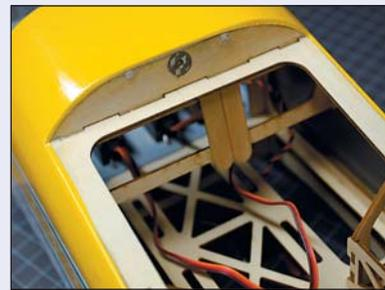
Spektrum's AR6100 is a two-part receiver. The main component is installed in the RC bay, but HM's editor wanted the sub-component to ride at a 90-degree angle to the main. A popsicle
