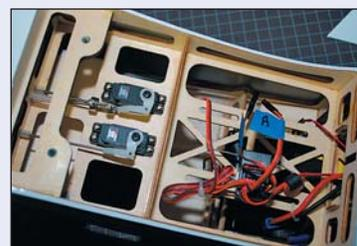
E-flite's Piper Pawnee 15e has plenty of room in the RC bay above the wing. Two JR SPORT MN48 servos are in there for the rudder and elevators. The main component of the Spektrum two-part AR6100 receiver
