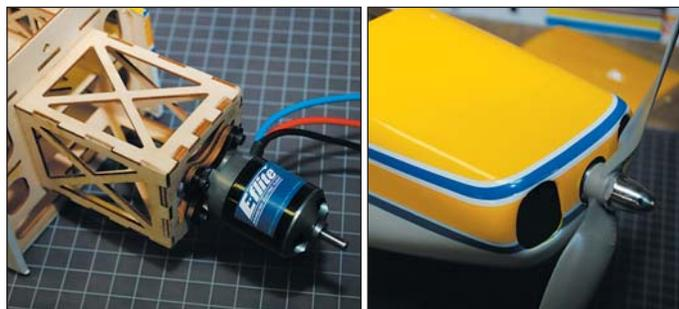
E-flite Power 15 is recommended for scale, and the sport setup calls for the Power 25 shown here. Beautifully factory-painted fiberglass cowl covers the motor and allows plenty of air entry and exit.
