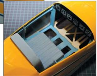
assure the correct mounting distance from the firewall so the propeller adapter and propeller will neatly clear the cowl.
