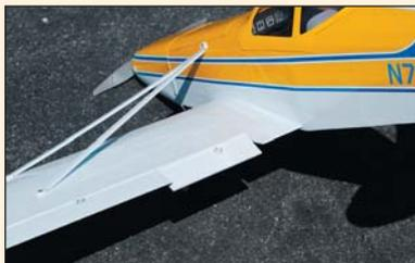
model, the end points for neutral and extended flap positions are adjustable mechanically or through programming.
