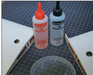
Pawnee wing is a two-panel affair that's easily joined with Hangar 9 slow-setting 12-Minute or 30-Minute Epoxy. A two-part, laminated plywood wing joiner sets the wing's dihedral angle. Apply adhesive and hold panels with blue masking tape until the epoxy fully cures.
