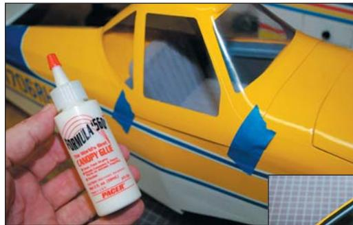
Semi-scale cockpit details include a mock velour ribbed pilot's seat and a good looking instrument panel. Use Pacer Industries' Formula 560 Canopy Glue to secure the big, factory-painted canopy over the 'pit.
