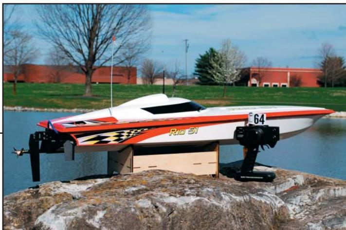
Not included but suggested items to assemble and run the Rio 51 are a 5.5mm nut driver, 7mm nut driver, 3mm hex driver, #2 Phillips screwdriver, #2 slotted screwdriver, 10mm wrench, a small personal retrieval system (we use the AquaCraft Atlantic Harbor Tugboat), 12 AA batteries, a gasoline jug, 2-cycle oil, mixing cups and funnel, GrimRacer 50 weight cable oil and GrimRacer Speed Grease drive lubricant.
