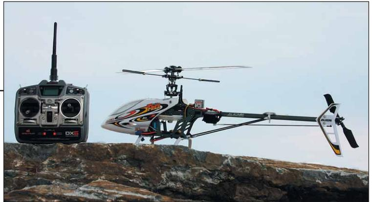
The quality of the parts and fit is immediately apparent. The links are sized correctly and move freely, and the aluminum head block, head button, tail boom and frames are nice touches that greatly improve performance over plastic because of their greater rigidity. The T-Rex is slightly larger than most electric micro helicopters, which also helps it to fly a bit more smoothly and take the wind
