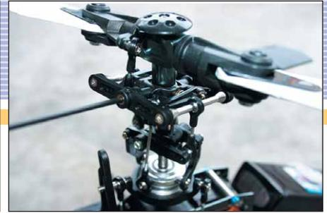
*Top-shelf mechanics, aluminum head block and 325mm PO wooden blades assure top performance from Align's new T-Rex 450SA ARF. Align's RCE-500X Heading Lock Gyro features remote gain from extra transmitter channel. It's very effective, and holds the tail solidly.*
