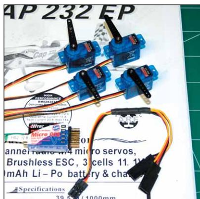
*Jeff Troy's model flies with the Micro 055 Receiver and four HS-55 servos from Hitec RCD.*
