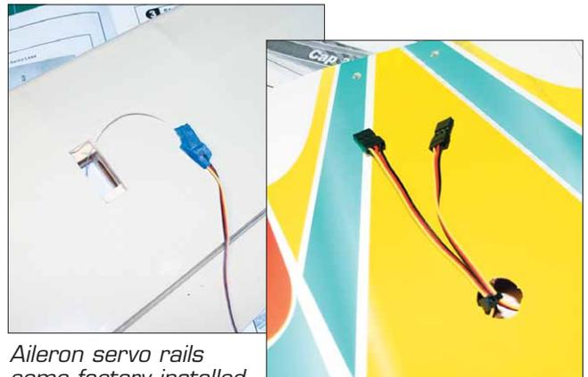
*Aileron servo rails come factory installed in the CAP 232, and their nearness to the wing centerline means that servo extensions are not required. Just use a Y-harness from the receiver.*
