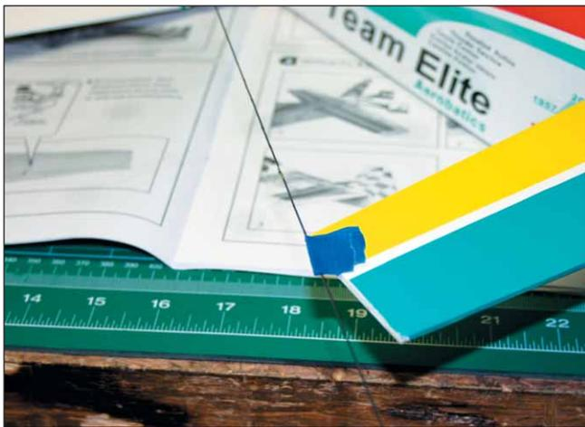
*Horizontal stabilizer slides through slot in fuselage. After centering the stabilizer, Jeff Troy uses a length of radio dial cord from the center of the firewall to assure the equal distance of both leading edges.*
