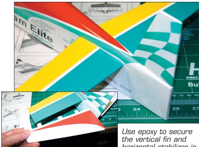
*Use epoxy to secure the vertical fin and horizontal stabilizer in the slots at the rear of the fuselage, then attach the elevator panel and rudder hinges with thin CA.*
