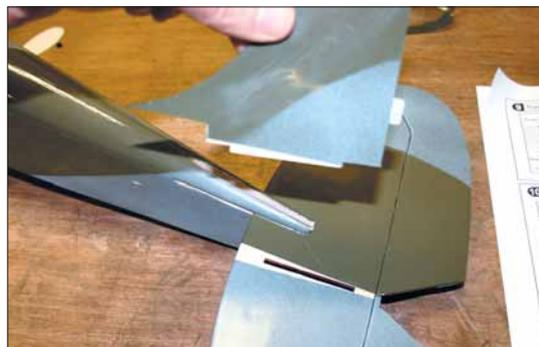
*Horizontal stabilizer and vertical fin interlock at rear of fuselage. Slots assure alignment.*
