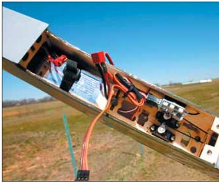
*RC bay shows JR Sport 6UL receiver and ST15 servos, AirBorne TWM Li-Poly battery and lead from AirBorne's new Brushless ESC. Y-harness to an ST15 servo in each wing panel operates ailerons.*
