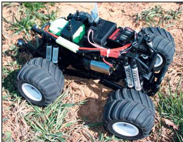
Small truck, but big features that include six-point ladder bar suspension, 4WD, mirror diffs and eight rugged shocks.
