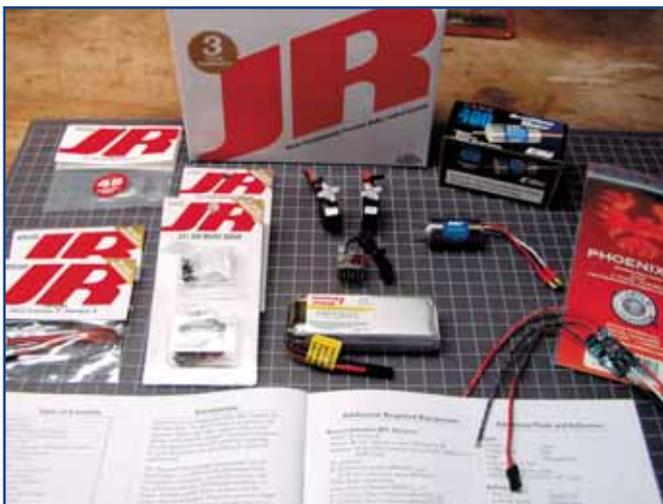
Extras include JR's Airpack Micro, extra 241 sub-micro servos and long servo arm sets, an E-Flite Park 400/4200KV brushless motor, Thunder Power 3-cell Li-Poly battery and a Phoenix-25 brushless/Li-Poly electronic speed control from Castle Creations.
