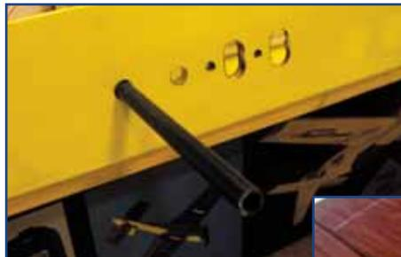
*E-Flite's Mini Funtana uses a rugged carbon fiber wing joiner, and the one-piece carbon fiber landing gear provides a sturdy mounting point for the model's painted fiberglass wheel pants.*
