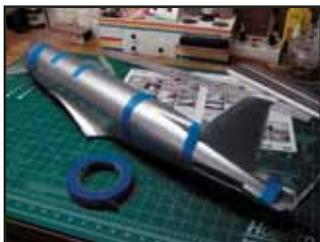
*The Skytrain's primary airframe components come factory painted in silver or olive drab. Drafting tape or Scotch 3M Blue masking tape is recommended to prevent marring the painted surfaces during the model's assembly. GWS Cement is included for general construction, although quick-setting epoxy is recommended when assembling the wing's outer panels to the center section.*
