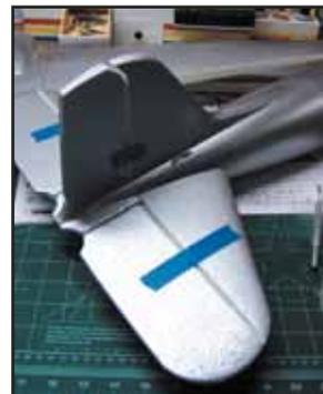
*Paper-like hinges are installed in control surfaces with GWS Cement, then attached to flying surfaces and secured with tape until glue is thoroughly cured.*
