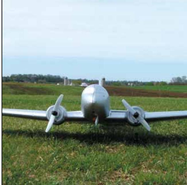
This kit builds very easily, and only a minimum of equipment, tools and supplies are needed. Most of the model's assembly is done with the included tube of GWS cellulose adhesive, and quick-set epoxy handles the rest. Required tools are limited to a razor knife and fresh blades, a needle-nose pliers, a ruler, a small drill and pin-vise, and a roll of drafting or similar low-tack tape.
