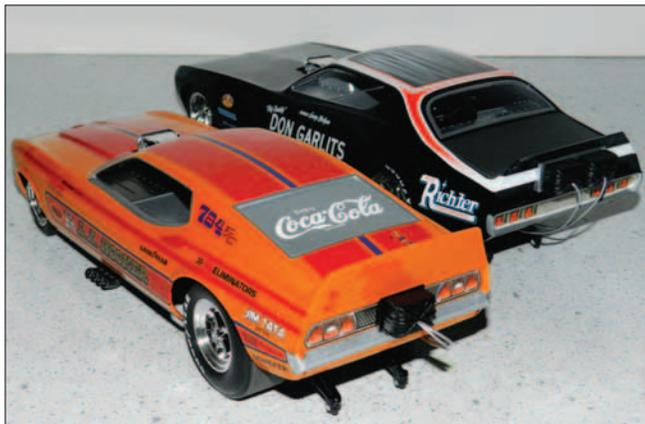
Both cars include a drag chute which is used to slow the car down at the end of a high-speed run.
