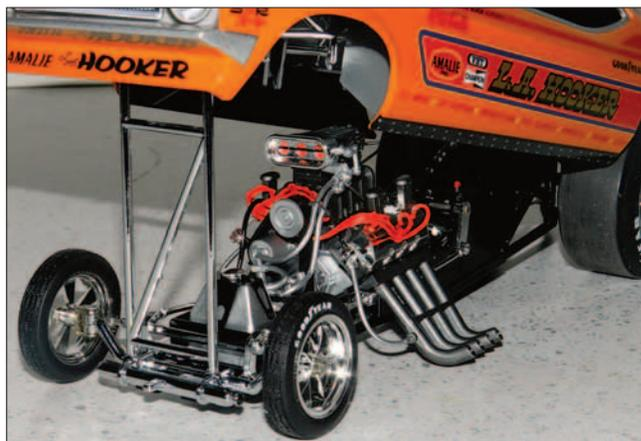
The front suspension is fully articulated, including the wheels which steer from the driver's position.
