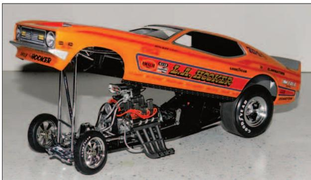
*There are no doors on a funny car. The body tilts open and is held in this position by a brace.*
