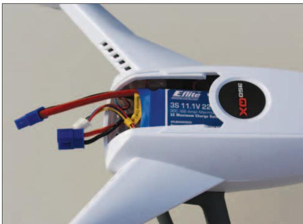
*The 350QX includes a 3S 11.1Volt 2200mAh lithium battery that fits securely in a molded tray.*
