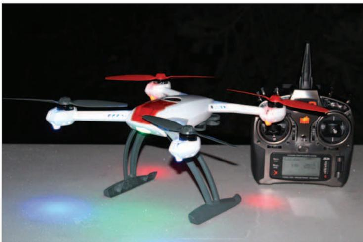
*With LEDs attached to each of the arms, blue for the back, red indicating the front, flight orientation is easily managed.*
