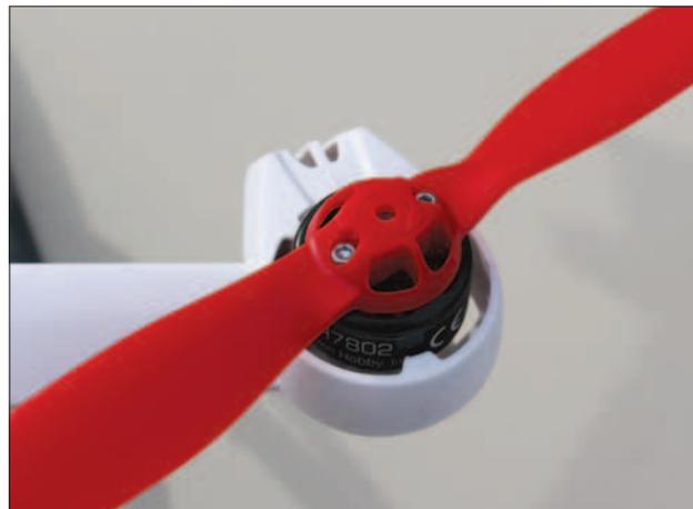
*The rotors are mounted directly to the motor, eliminating the need for any type of prop adaptor.*
