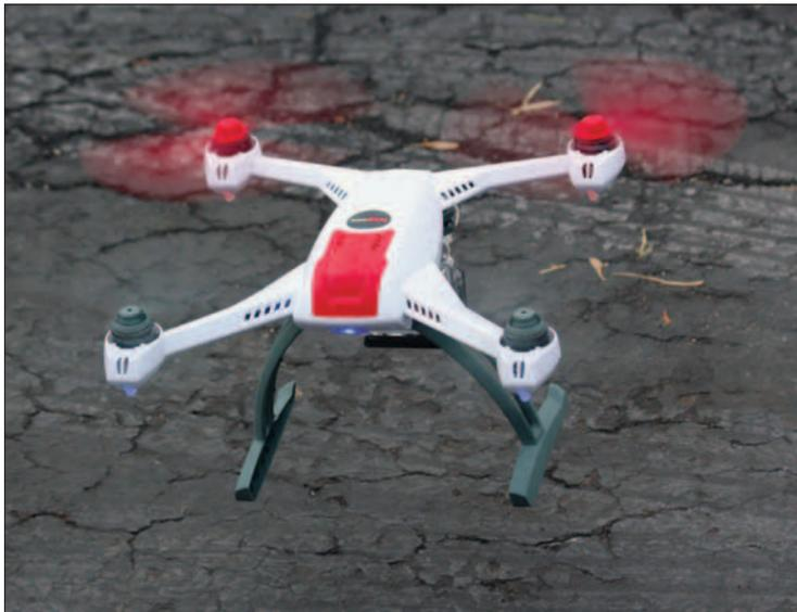
*Caught on lift-off, the blue LED directly under the red hatch cover indicates the 350QX is locked in the Stability Mode.*
