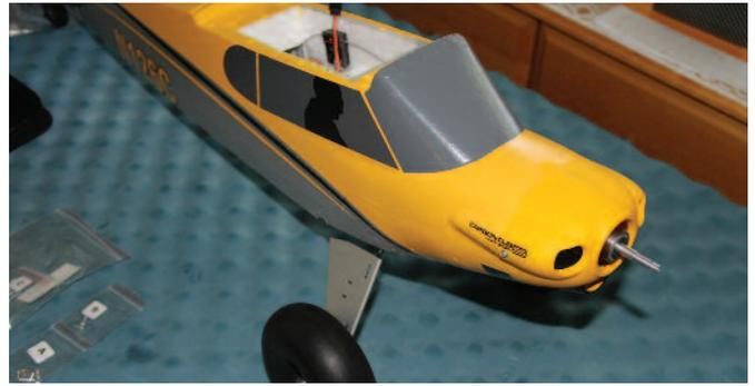
*When assembling any electric powered aircraft the final step involves the mounting of the propeller. Stress to the purchaser the need to comply with this step. Too many aircraft have been damaged and too many modelers have suffered minor injuries that could easily have been prevented had the propeller been left off until it was needed.*
