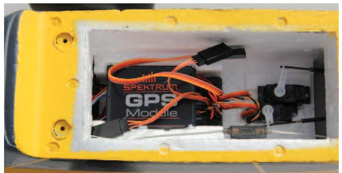
*Just about every bit of space in the equipment compartment is fitted with a piece of electronics needed to assure the end user's success. This includes the elevator and rudder servo, the receiver, which is mounted to the fuse side, a GPS module used for securing the location of the aircraft, and beneath the GPS is a stability module used to keep the aircraft level during flight.*
