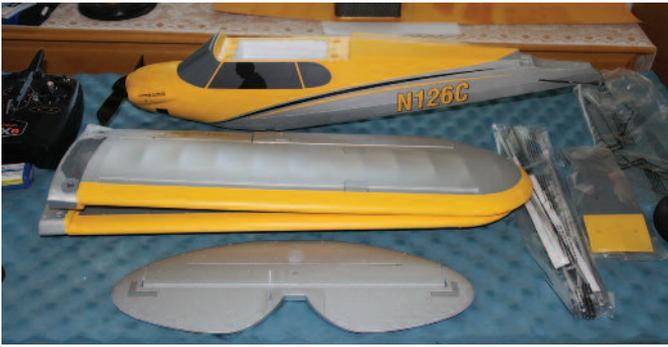
*As in all models of this class, the Carbon Cub 1.3 is shipped as a basic kit that needs to be assembled by the end user. At first glance it may seem complicated especially to the new enthusiast, but when broken down into individual assemblies, it's the landing gear, wing and tail. All told, about two hours worth of relaxed building is required.*
