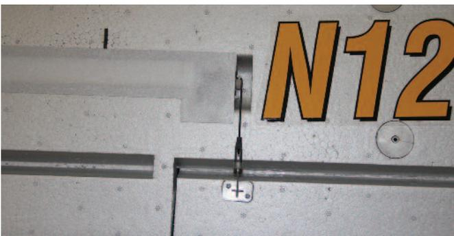
*Individual aileron servos result in short and direct links to the ailerons. In the case of the review aircraft no mechanical adjustment to the aileron linkage was necessary, but if it is needed simply remove the clevis from the horn and adjust the clevis in or out as necessary on the threaded rod.*
