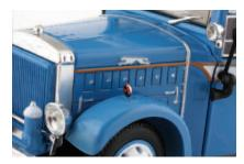
The chromed theme continues on the hood with plated handles and fasteners. individual studs or knobs on the six 'flipflap' engine vent shutters fitted to each of the hood's side panels, plus the 'sprinting greyhound' logo in plated relief.
