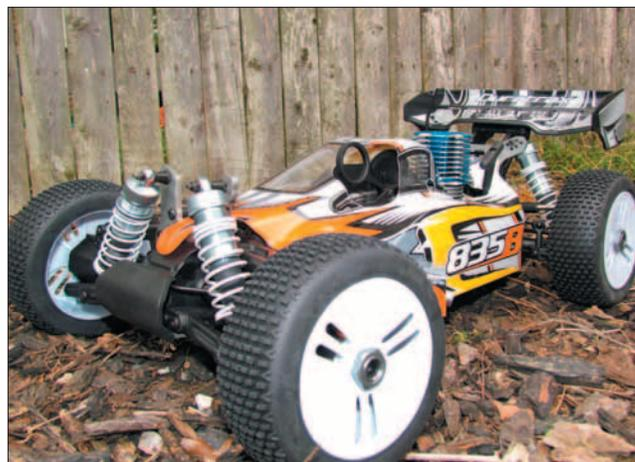
high end parts to be found. Big bore aluminum oil filled shocks, aluminum shock towers, aluminum axle carries and torsion bars are all included. What I like is Duratrax did not go overboard with machined aluminum. Too much metal in a suspension system can lead to massive damage as a result of an unplanned impact.
