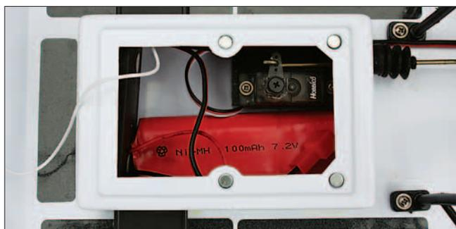
*The radio compartment is compact and simple in layout. Included is a 1100 mAh NiMH battery that can be upgraded in capacity and voltage for enhanced performance.*
