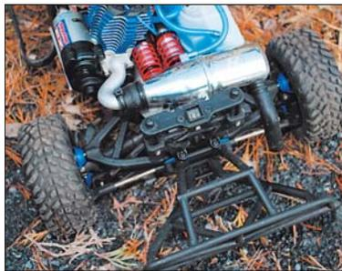
powerplant gets the Slayer moving in a hurry and keeps it out in front. Helping the TRX 3.3 achieve its maximum power is an aluminum Resonator tuned pipe. The pipe's highly polished finish, as well as the engine's attractive blue-anodized head, gives the Slayer a custom look.
