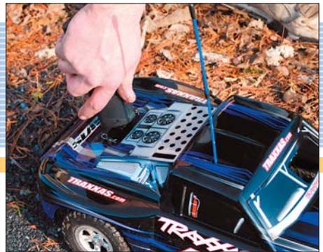
Lid-off view shows Traxxas 3.3 engine, tuned pipe and EZ-Start unit. Fill the tank with Traxxas Top Fuel, insert the EZ-Start hand-held starter, push the button and get ready for the ride of your life. Traxxas' engine starts quickly and stays running — very fast!
