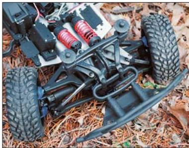
Slayer's four aluminum GTR shock absorbers ride inboard to protect against damage. Rugged front and rear bumpers absorb reasonable impact shock.
