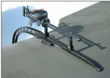
One-sixth scale Lewis Machine Gun from Williams Bros. rides atop the S.E.5a's upper wing. Gun mount is made from wood scraps, and the magazine reloading track is made from three pieces of
