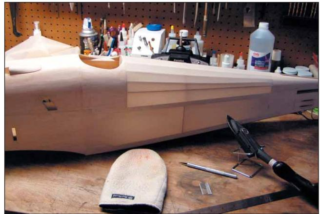
Super Coverite is so pliable and workable that the British Scout's fuselage top and sides are covered with a single piece of fabric. Bottom is separate.
