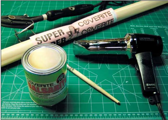
Finishing products used for the S.E.5a from the Coverite line include Super Coverite fabric, Fabric Formula Balsarite and the 21st Century Iron.
