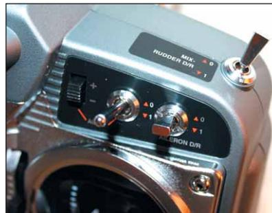
*DX7 control switches are in traditional locations. Left side of the transmitter case has toggle switches for elevator rate, flap mixing and landing gear. Aileron rate, rudder rate and Auxiliary Channel 2 are on the right side.*
