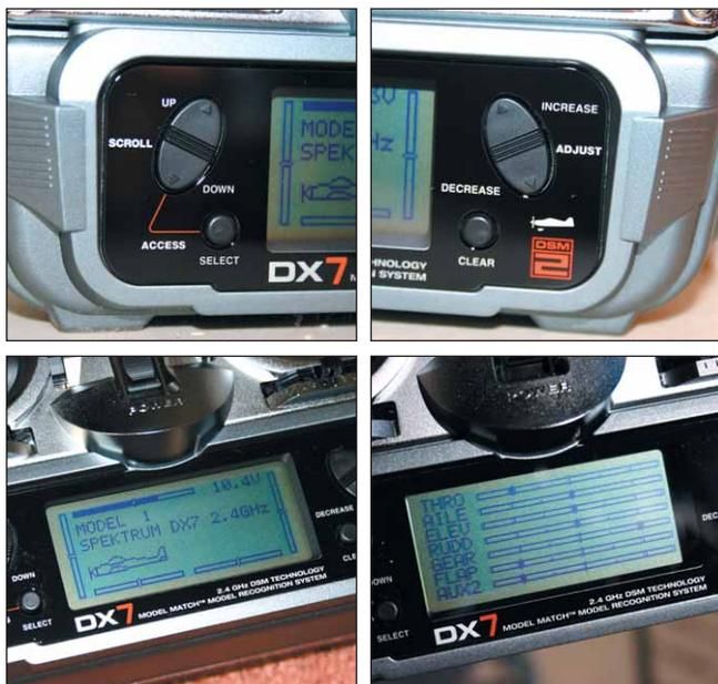
The DX7 menu is accessed and handled with only two rocker switches and two touch buttons. Dual frequency selection is automatic and happens every time the system is turned on. The chance of any two fliers being on the same two frequencies (of approximately 2 billion available) is virtually impossible.
