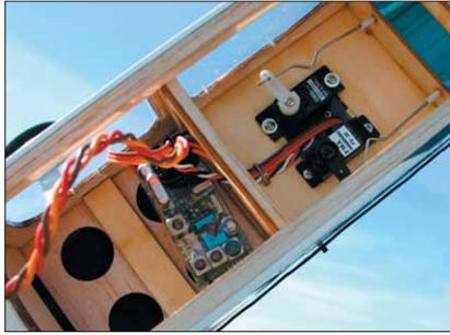
*HM's review model uses FMA's eXtreme 5 receiver, two FMA PS30 servos for ailerons and one for rudder, and GWS servo for elevator.*
