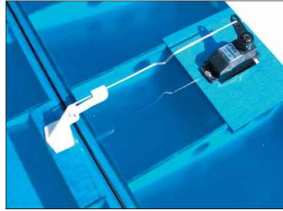
5/8" down. I wasn't sure if each entire line was crossed or just the up-down/right-left parts, so I split hairs and set both surfaces for 1/4" deflection in each direction.
