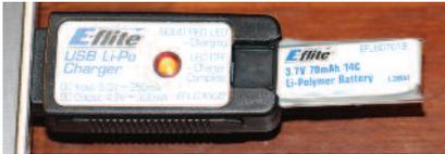
Included with the Vapor Lite HP is a USB style charger and a 3.7V 70mAh flight battery.
