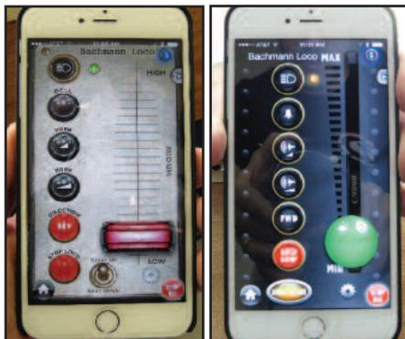
*There are different control panels available for the user to select from each working exactly as a standard hard-wired controller.*
